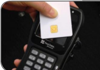
**Contactless card reader** — The contactless card reader antenna is embedded behind the display and PIN pad. The reader's lights will show blue when the PIN Pad is powered on to indicate the reader is working normally. To process a contactless payment, place the contactless card near the card reader antenna during a transaction.
