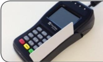
**Magnetic card reader** — The card reader slot is on the right side of the PIN Pad. With the magnetic stripe facing [inwards], slide the card in either direction through the slot without stopping. If the card swipe fails, check the position of the magnetic stripe and slide the card again.
