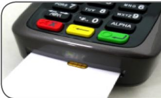
**Smart card reader** — The integrated circuit card (ICC) reader is located at the bottom end. Please make sure that the gold ICC contact pad is facing upward when inserting the card into the slot.
